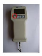
**2.** When display shows zero, simultaneously press "UNIT" and "ZERO" button until "CAL" appears on display.
