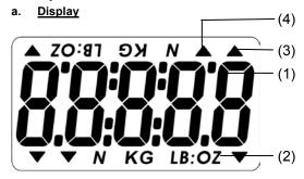
Measuring Result Measuring Units Measuring Direction Indication of PEAK Mode
