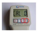
**3.** Wait a few seconds and display will show the necessary adjustment weight, e.g. 5,000kg for FK 50 or 10,00kg for FK 100.
