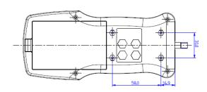
Fixing by 4 x M3 screws.
